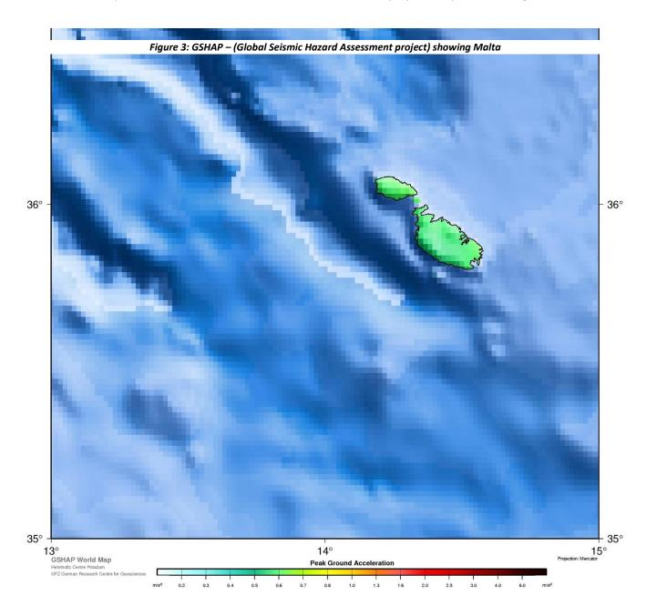
*Figure 3* notes peak accelerations as varying from  $0.7 \text{m/s}^2$  down to  $0.55 \text{m/s}^2$ , with the south eastern cliff face being the more stable location. The above ground acceleration values note the Maltese Islands according to EC8 to be classified for low seismicity.
