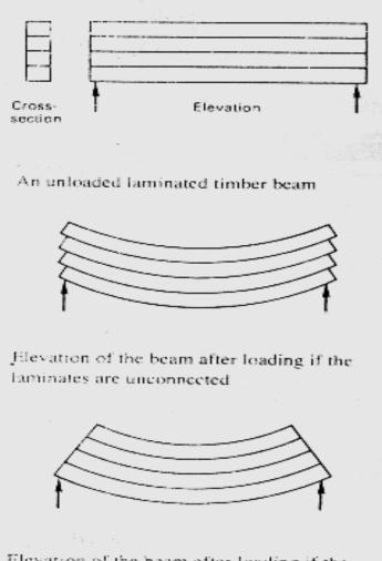
Elevation of the beam after loading if the laminates are securely bonded
