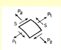
Membrane stresses are under equilibrium due to direct and shear forces only due to geometrical curvature. Compressive forces introduce the concept of buckling.
