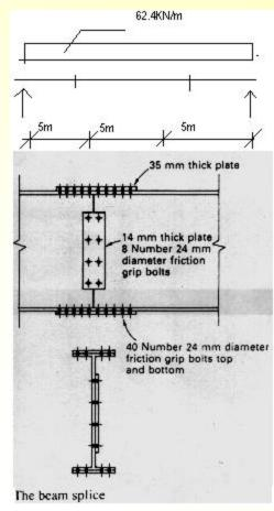
No of flange bolts 1825KN/102KN = 17.9(say 20 per side) No of web bolts 156KN/102KN = 1.5 (say 4 per side)
