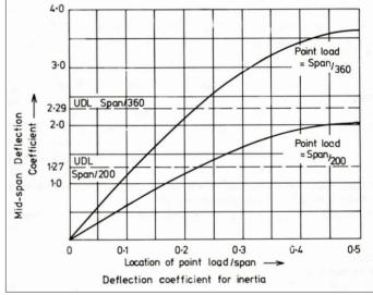
Deflection coefficient for inertia (reproduced courtesy of BCSA)
