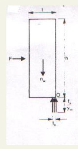
the design vertical load n<sub>w</sub> is resisted by a rectangular stress block of width t<sub>n</sub>
