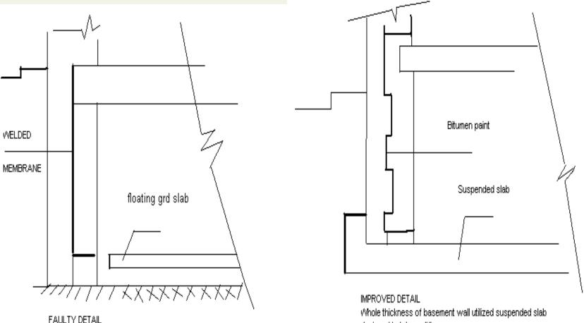
Basement wall acts as 2 separate skins. (no shear key) floating slab subjected to upward water pressure designed to take up lift
