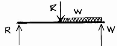
and no matter how the load  $W$  is altered in value or position, the right-hand reaction must always equal that load.
