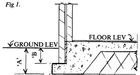
are within 0.5 m (1 ft 6 in) of the concrete surface'. Obviously, if the found thickness dimension A is greater than 0.5 m, it will protrude without cover. What minimum cover (dim. A) is therefore required with regard to normal frost conditions? The question does not refer to deep permafrost conditions or foundations where special precautions need to be taken against chemical attack.
