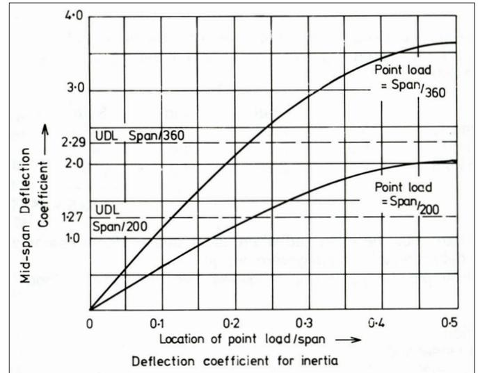
1 Deflection coefficient for inertia (reproduced courtesy of BCSA)
